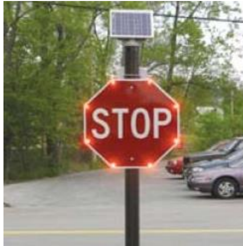
Example of a stop sign with embedded LEDs and solar unit
